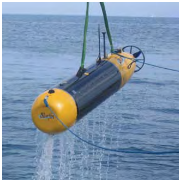
A Bluefin-12 Autonomous Underwater Vehicle (AUV) captures continuous, real-time information on ocean conditions
